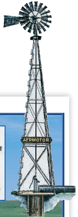
STEEL WINDMILL In regions of unpredictable rainfall, the steel windmill prevented crop dehydration by bringing up underground water for irrigation.
